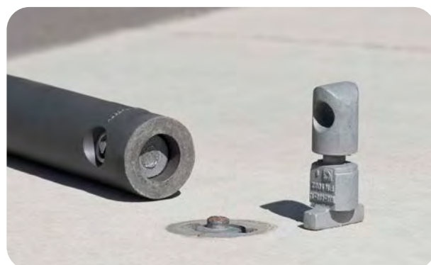
The replaceable connecting piece breaks at the predetermined breaking point. The bollard and foundation with ground shell usually remain intact.
